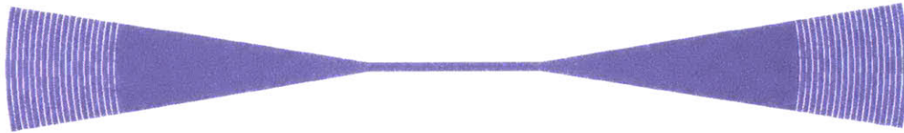
Figure 5-2: Structure for testing waveguide loss.
