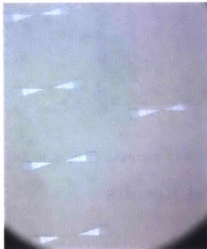
Figure 5-6: 50x microscope image of structure for testing waveguide loss.
