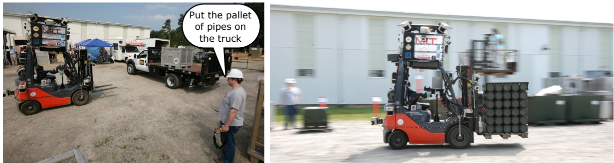
Figure 1: (left) The mobile manipulation platform is designed to safely coexist with people within unstructured environments while performing material handling under the direction of humans.
