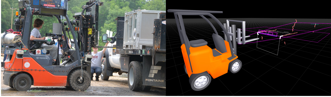
Figure 7: The robot detects the presence of the truck bed and pallet and maintains estimates of their geometry throughout engagement using LIDARs mounted to the tines and carriage.
