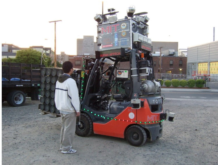
Figure 16: The robot utilizes a combination of LED signs and LED lights to indicate that it is aware of people in its vicinity. The lights mimic the robot’s gaze towards approaching pedestrians.
