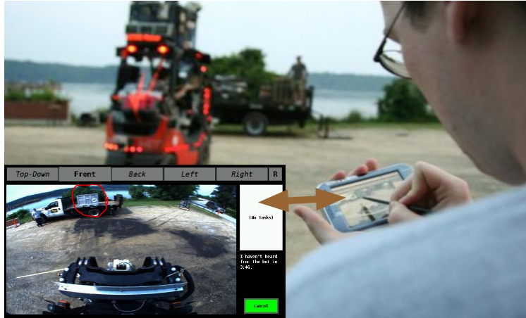
Figure 13: The handheld tablet provides one means for the user to interact with the robot. The tablet enables the user to visualize the robot's situational awareness and to convey task-level directives through a combination of pen-based gestures and natural language utterances.
