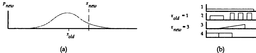
Figure 13 The mutation operators. If selected for mutation, a time was mutated by applying Gaussian noise to the existing value (a). An execution mode was mutated by replacing the current mode with a different mode from the set of modes for the corresponding task (b).
