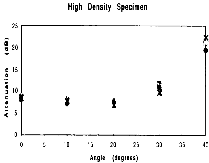
Figure 3-4 The attenuation vs. Angle plot for the high density specimens
