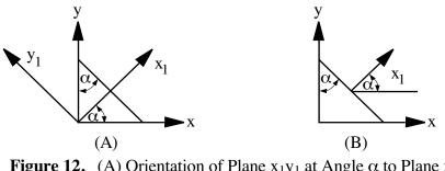
Figure 12. (A) Orientation of Plane x<sub>1</sub>y<sub>1</sub> at Angle α to Plane xy;(B) Wedge for Equilibrium Analysis.
