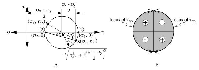
Figure 13. (A) Mohr's Circle of Stress; (B) Shear Stress Sign Convection for Mohr's Circle.\*
