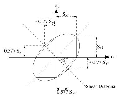
Figure 30. Failure Locus for the Biaxial Stress State for the Maximum Distortion Energy Theory
