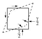
Figure 10. State of Pure Shear Strain
