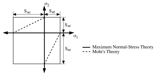
Figure 24. Failure Locus for Mohr's Theory
