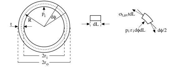
Figure 19. Radial Forces in an Internally Pressurized Thin-Walled Cylinder.
