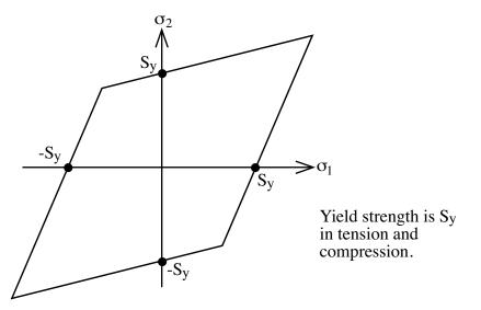
Figure 29. The Failure Locus for the Maximum Normal Strain Theory (for fixed v).
