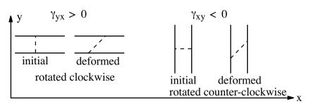
**Figure 9.** Strains resulting from Shear Stresses  $\pm \gamma_{xy}$ .
