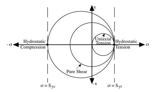
**Figure 22.** Principal Mohr's Circles for Several Stress States Representing Incipient Yielding According to Maximum Normal Stress Theory (Note, for Pure Shear  $\sigma_1 = |\sigma_2| = \tau$ ).
