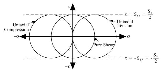
Figure 25. Stress States for Yielding According to the Maximum Shear Stress Theory
