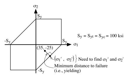
Figure 35. Maximum Shear-Stress Theory
