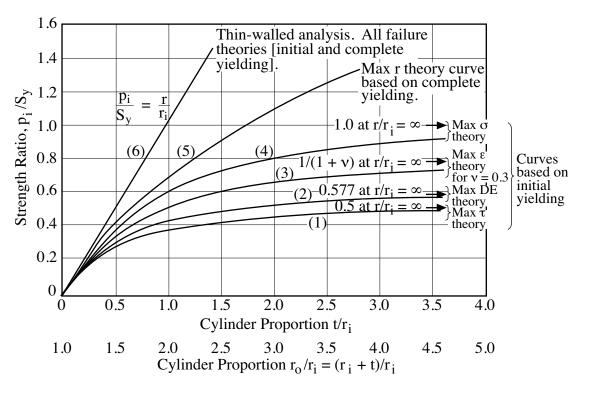
Figure 33. Failure Predictions for Internally Pressurized Cylinder
