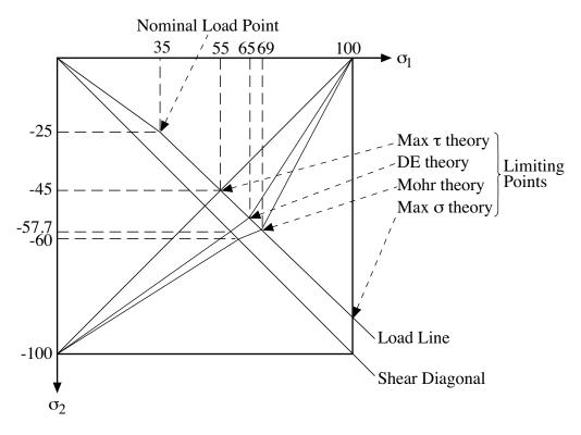
Figure 36. Failure Theories for Example 2 Conditions
