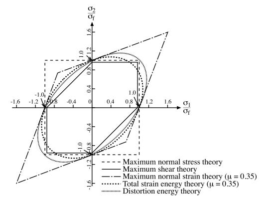
Figure 31. Comparison of Failure Theories for a Biaxial State of Stress. (From Ref. 4, p. 123.)
