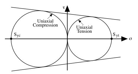
Figure 28. Mohr's Failure Theory for Uniaxial Tension and Compression
