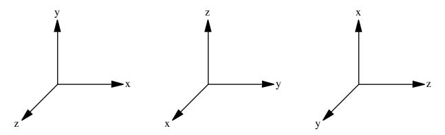
Figure 2. Right-handed System of Rectangular Coordinates.
