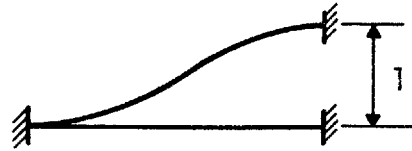
Fig. II-9 Influence Line for the Vertical Reaction of a Fixed End Beam
