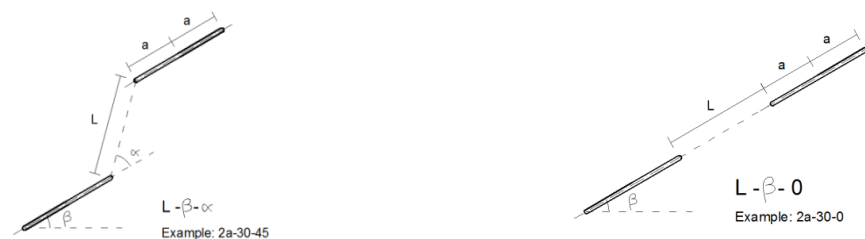
a) b) Fig. 1 Parameters used to describe double-flaw a) stepped and b) coplanar geometries. L is the ligament length, which is the distance between inner flaw tips expressed in terms of half flaw length a=1/4 inch in the current study; \beta is the angle that the flaws make with the horizontal; \alpha is the angle that the direction of the ligament between inner tips makes with the axes of the flaws. \alpha is zero for coplanar geometries
