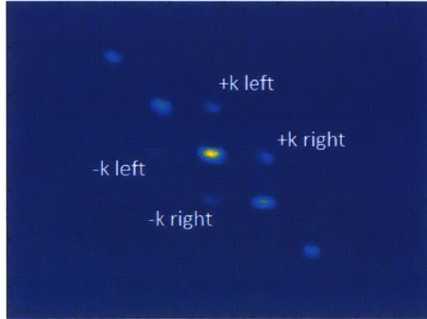
Figure 4-25: A typical time-of-flight image in the spin-orbit coupling experiment, and the notation used in our data analysis. The relevant peaks are explained in the text.
