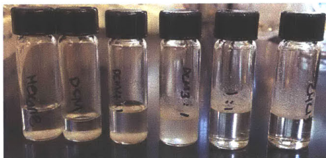
Figure 2-15. PDMAPS ( M_n 67,360, PDI 1.051) powder in various mixtures of organic solvents. From left to right, hexane (0.659), dichloromethane (1.326), 4:1 volume mixture of dichloromethane and chloroform (1.363), 3:1 volume mixture (1.378), 1:1 volume mixture (1.41), and chloroform (1.4788). Densities are indicated in parentheses.
