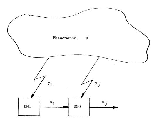
Figure 2: Two DM Tandem Topology
