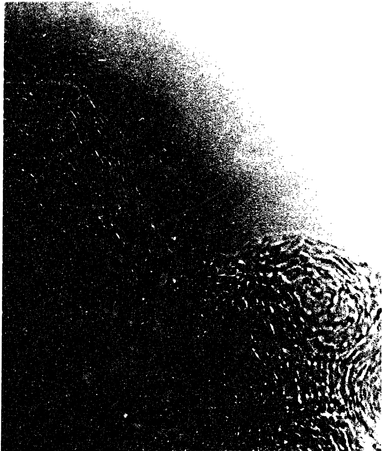
Figure 1-4: High resolution transmission electron micrograph image of a soot particle collected from the atmosphere in Cambridge, MA.
