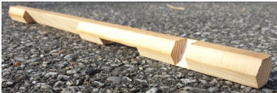
Fig. 15.5. The Hex Reducer. This design of an entrance reducer uses a hexagon for the cross-section. This hexagonal shape allows three unique sizes to be made instead of two, improving the functionality of the entrance reducer. Additionally, its iconic shape can make it attractive to beekeepers.
