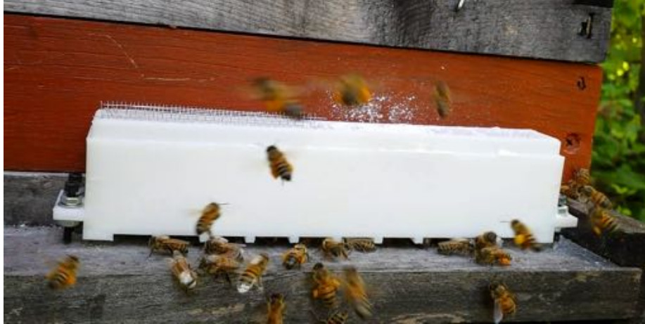
Fig. 15.2. Testing of the Varroa Prototype showed that the sugar could be localized on the backs of the bees. Sugar did land on the backs of the bees with some on the wings. Over time less sugar was noticeable on the wings of the bees.
