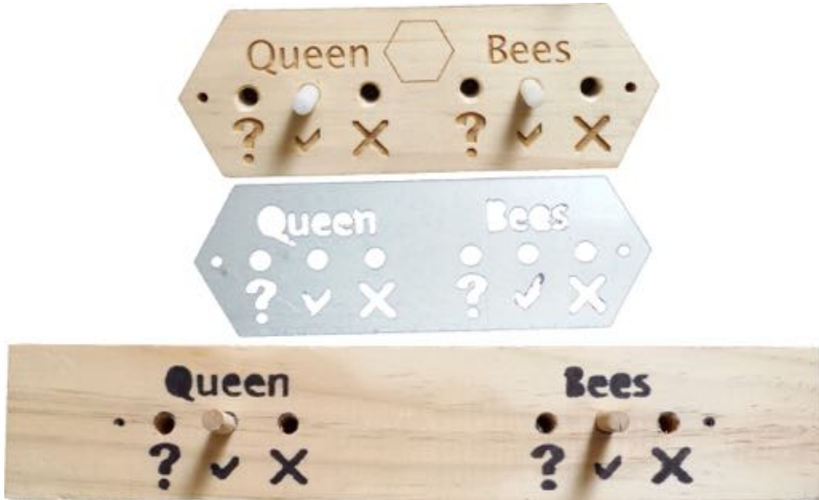
Fig. 14.4. Peg and hole design. This design for improving hive management started with a hexagon inspired flat plate that could easily be placed on the hive. The concept was to make it easy to place the small pegs in an easy-to-understand design. Recognizing that for replication, the words and symbols needed to be made faster, a stencil was made and a longer piece of wood that could also serve as a hive handle was created.
