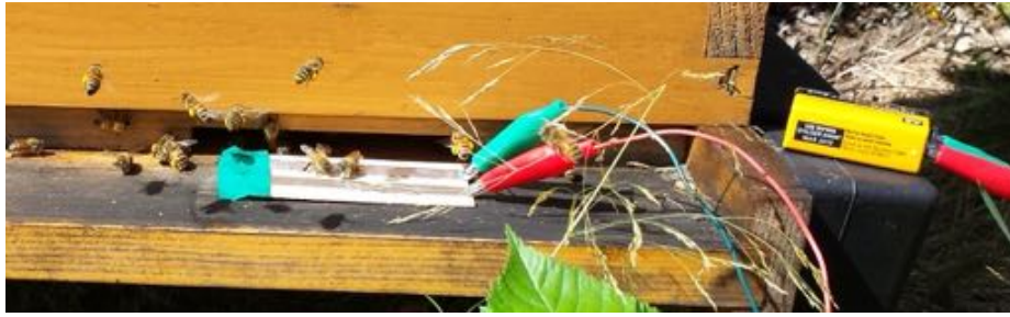
Fig. 10.3. Low voltage shocking of bees.
