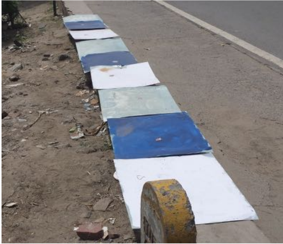
Fig. 12.9. Painted roof testing.
