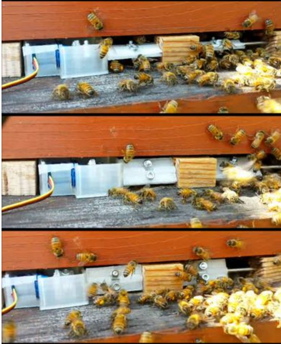
Fig. 8.4. Butterfly valve prototype testing. It was found that bees would not get stuck under the entrance if the entrance moved slowly enough. The above pictures show the entrance in the open state, during closing, and while closed. Note that the bees use both the upper and lower part of the entrance.
