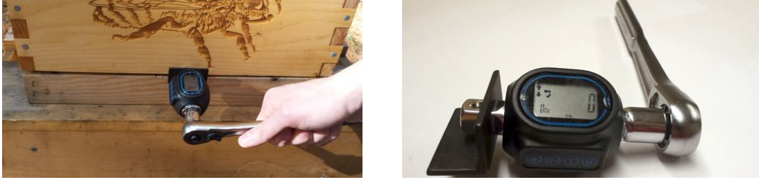
Fig. 5.4. One commercially available TWB design is the Nectar Detector. It has a 50.8 mm (2 inch) long right angle bracket mounted to a digital torque wrench.
