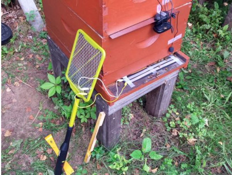
Fig. 10.1. Setup for prototyping a high voltage shocking method against wasps.
