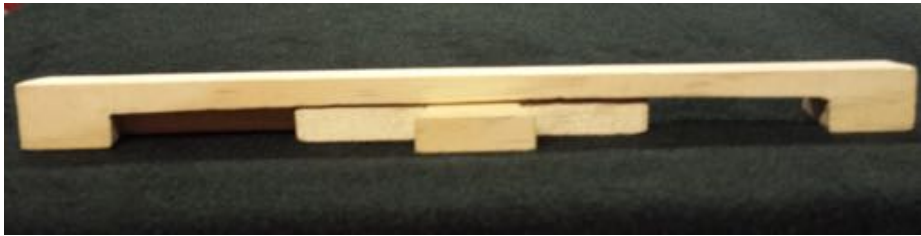
Fig. 8.8. Manual wedged slidable entrance.
