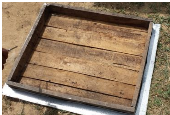
Fig. 12.6. Warped boards make air gap.
