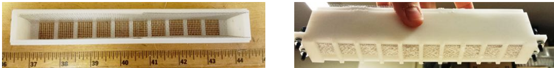
Fig. 15.1. Sugar depositing entrance prototype to counter varroa. This prototype was 3D printed and then filled with powdered sugar on top of a screen layer. The design was to have the hairs of bee backs dislodge the sugar that would coat bee backs, encouraging localized grooming. The grooming can help bees remove the varroa mites from each other. In practice the box would have a lid.
