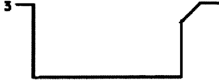
Figure 1.2: Cavity configuration with trailing edge ramp as assessed by Shaw [24] for mitigating cavity response in pressure fluctuation.
