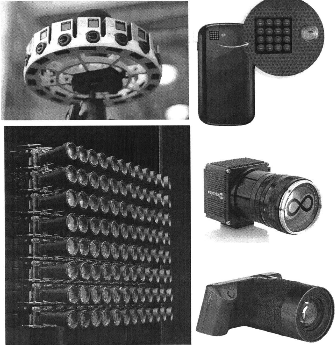
Figure 1-4: Light field imaging hardware implementations. Clockwise from top left: Google Jump 360 [32] degree circular camera array consisting of 16 GoPro cameras (credit: Will Shanklin/Gizmag), Pelican Imaging depth sensor array embedded in a cell phone [22], Raytrix [49] and Lytro [46] plenoptic cameras, respectively, and Stanford light field camera array [74].
