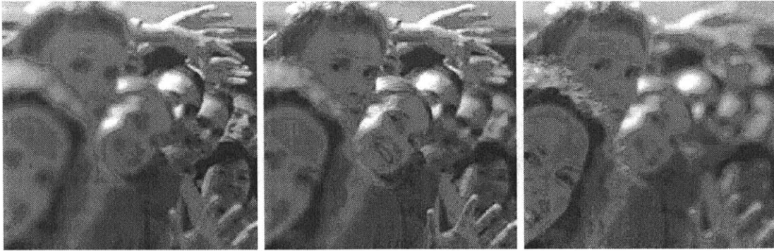
Figure 4-9: Refocusing an image volume at different depths using digital light field photography (reproduced from [45]).
