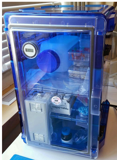
Figure 4.15: Secador vertical drybox cabinet used for storage of moisture sensitive materials, including A-PNCs, Nafion, IL and silica gel (51.8 H x 34.1 W x 41.4 D cm ).
