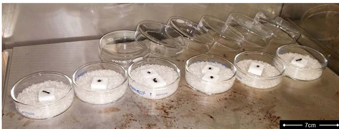
Figure 4.26: Ionic liquid batch infusion inside vacuum oven at 100 °C and 10 millibar . A-PNC samples situated in IL on teflon trays, placed inside glass petri dishes filled with silica gel.
