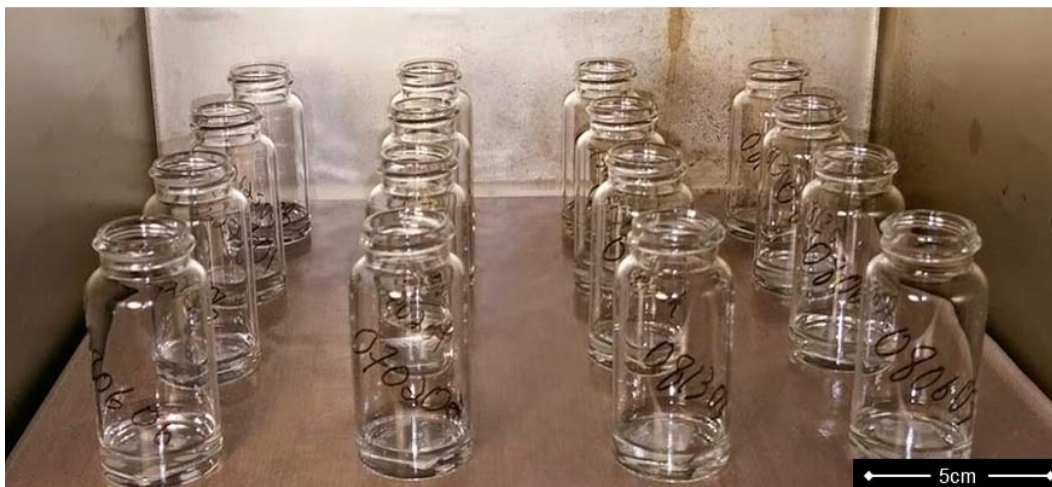
Figure 4.13: Nafion batch infusion into A-CNT process, showing 16 caged CNT systems in 20 mL glass vials inside vacuum oven. Vials are filled with Nafion in DMF solution, with the high vapor pressure of DMF allowing for a slow and high quality infusion.
