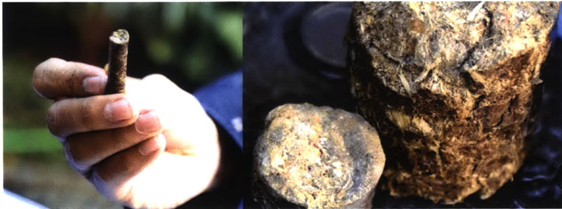
Figure 58: A sample of the pellets (left) and briquettes (right) generated by the pelletization process at Gangotree. Source of images: Kornstein, 2012.
