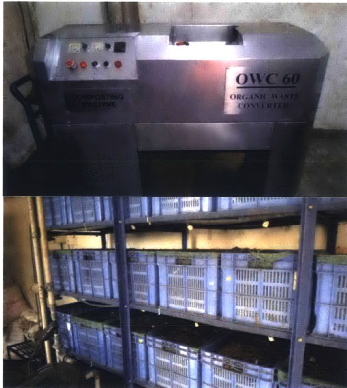
Figure 48: Organic Waste Converter (OWC) machine and curing compost that has been processed with the OWC.
