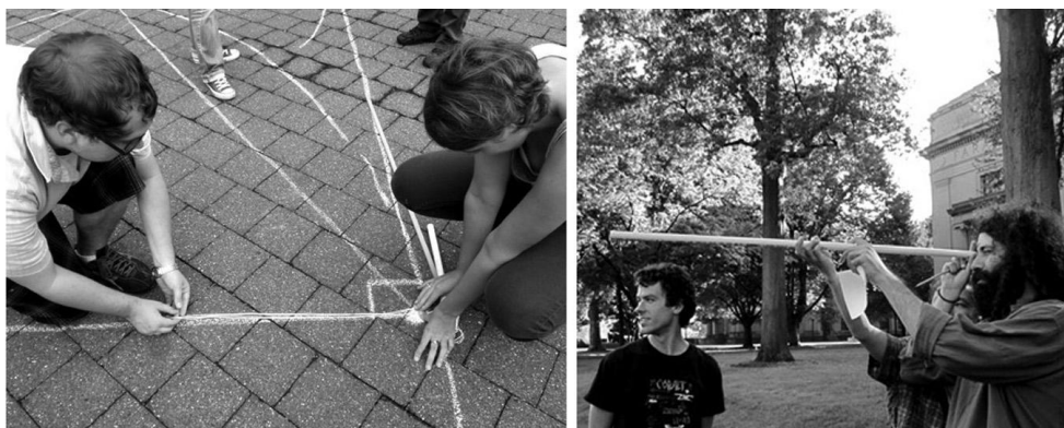
Figure 5. Left: Does the square's corner make a right angle? Students check whether the sides of a triangle formed from it obey the 3-4-5 ratio. Right: the observer of the outdoor square [left of photo] uses a tube to view it.
