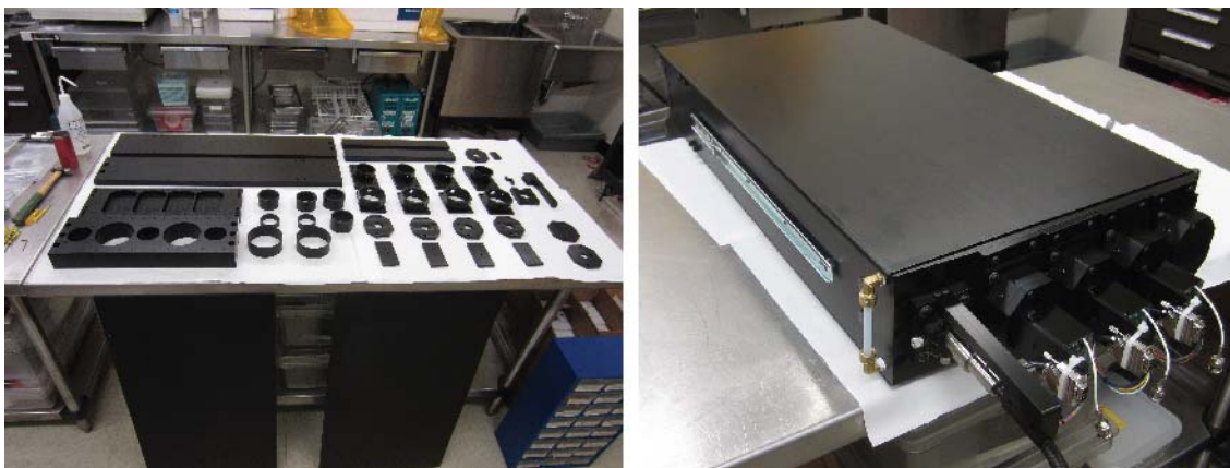
Figure 60: Photograph of the anodized prototype polychromator components prior to assembly (left) and fully assembled (right).
