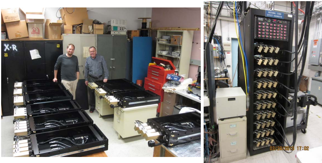
Figure 73: Photographs of the 10-sightline multi-spectral system during assembly. The 10 polychromators assembled in the lab with top covers removed (left) along with the author and his thesis advisor. The 10 polychromators with their control system assembled into the electronics rack in the MSE area of the C-MOD diagnostic hall (right).
