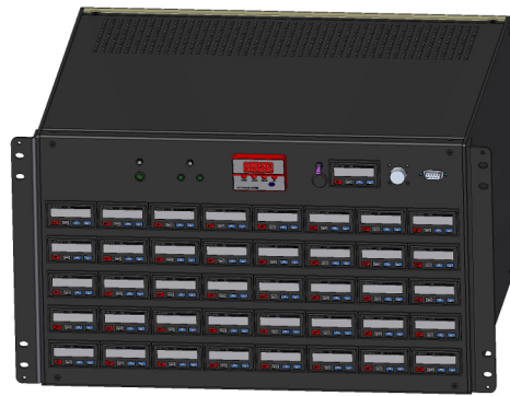
Figure 71: The polychromator control hardware with 40 oven controllers and APD gain control all commanded through TCP/IP.
