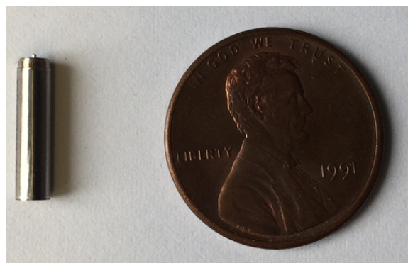
Figure 6-12: 3 mAh implantable medical battery from Quallion used in the implant.
