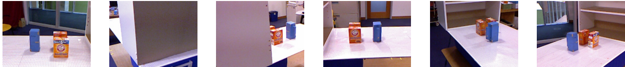
Figure 3-9: Examples of views from scenario 5. In all views except the final one, only one of the two orange baking-soda boxes was detected. This causes MHT to incorrectly infer that all measurements came from a single object (and prune other possibilities), whereas batch approaches such as clustering can revisit previous associations and correct them using new information, such as the final view where both boxes are finally detected.
