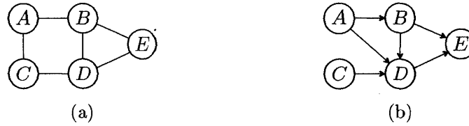
Figure 2.1: (a) Undirected graphical model example: P(A, B, C, D, E) \propto f_1(A, B) f_2(A, C) f_3(B, D) f_4(C, D) f_5(B, D, E) . (b) Directed graphical model example: P(A, B, C, D, E) = P(A) P(B|A) P(C) P(D|A, B, C) P(E|B, D) .
