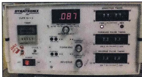
Figure 4-11: The electroplating current controller.
