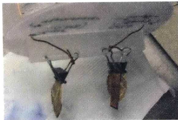
Figure 4-13: Image of the sample holder when a sample is clipped in.
