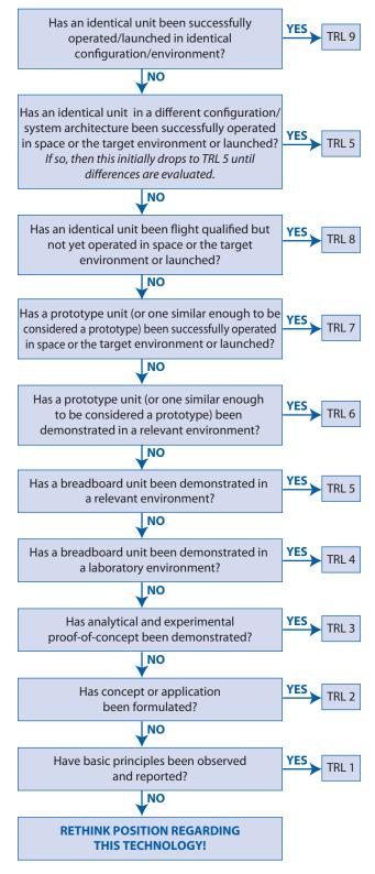
Figure G-5 The TMA thought process
