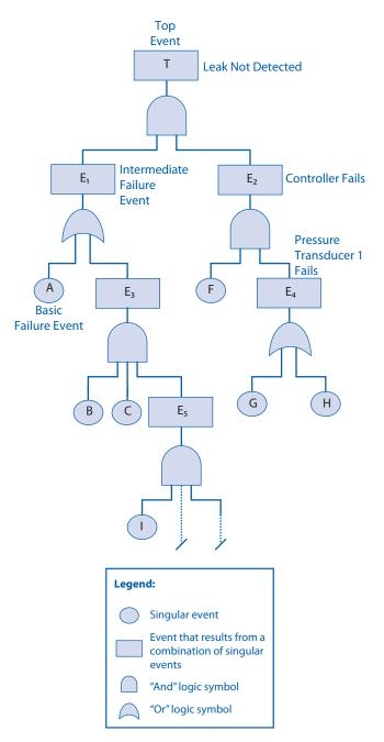
Figure 6.4-8 Example of a fault tree
