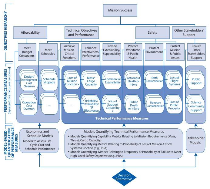
Figure 6.8-10 Example of an objectives hierarchy
