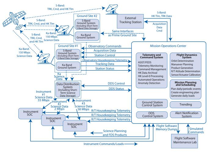
Figure 4.1-4 Example of an associated end-to-end operational architecture
