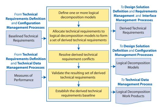
Figure 4.3-1 Logical Decomposition Process
