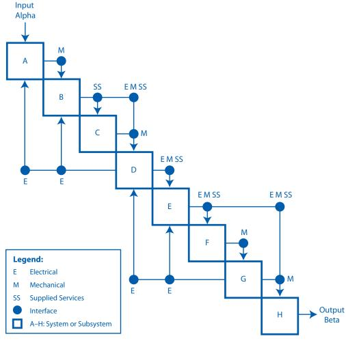
Figure 4.3-4 Example of an N2 diagram
