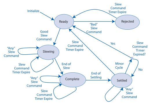
Figure F-8 Slew command status state diagram
