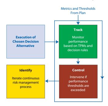
Figure 6.4-10 Performance monitoring and control of deviations
