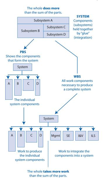
Figure 6.1-4 Relationship between a system, a PBS, and a WBS
