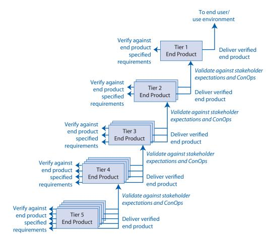
Figure 5.3-2 Bottom-up realization process
