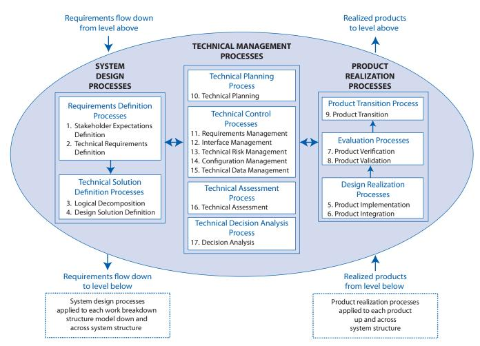
Figure 2.1-1 The systems engineering engine
