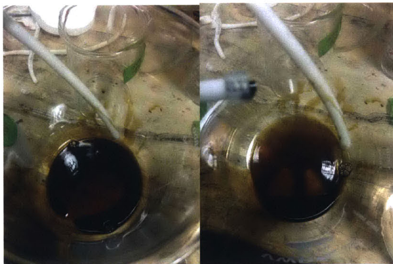
Figure 6-26: At the end of the concentrating feed run, the concentrated black liquor was collected from the retentate line (the white tube in the picture) into the beaker below. The concentrated black liquor from the retentate stream can be seen in the beaker. Strong viscosity and thickness of the solution can be observed in the pictures.
