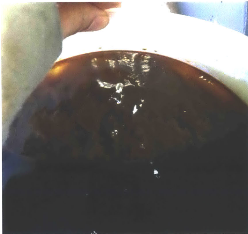
Figure 3-12: Traces of deposited lignin and other solids at the bottom of the fresh black liquor container
