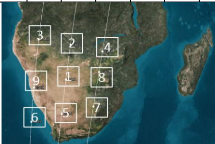
Figure 21: Eight available differential RAAN-TA slots (exact values in Table 1) arranged around the reference satellite (+1), as enumerated in an AGI-STK simulation.
