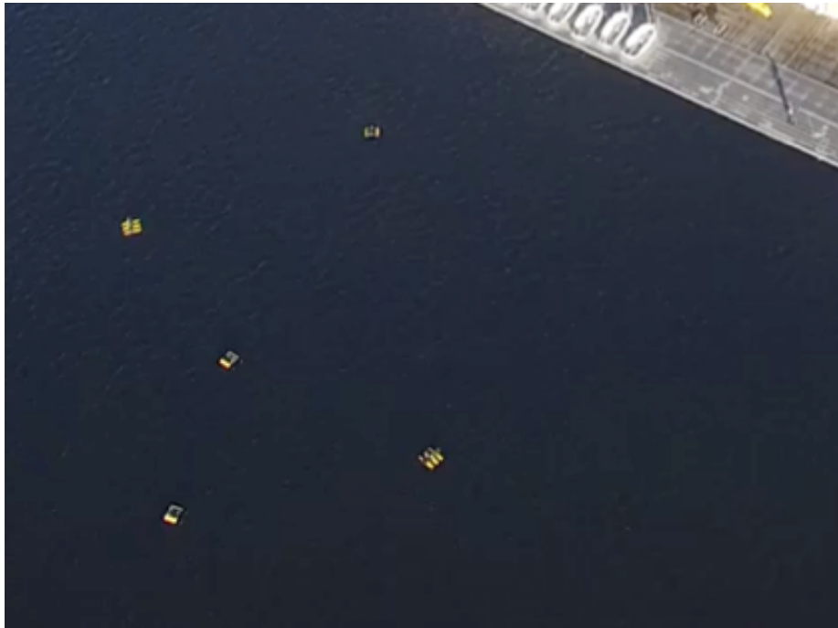
Figure 6-10 Vehicles were allowed to operate in close proximity to each other during Scenarios H-J as shown here. Prioritization of when to make collision avoidance decisions relative to the time of contact detection greatly influenced safety and protocol compliance results.
