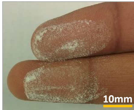
Figure 2.11 Baking soda was used to mark the contact area of the skin on the fingertips with the thermal display.
