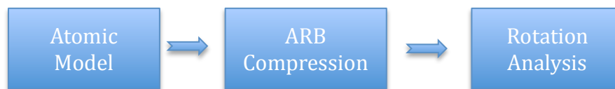
Figure 2: Three stages of experimentation. Building a model, compressing it, and analyzing compressed structure
