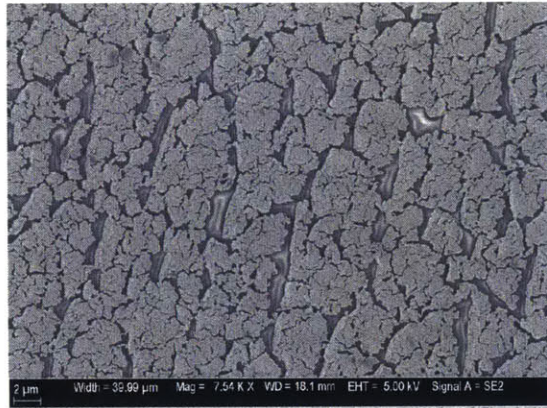
Figure 2-3: Morphology of 100nm gold thin film deposited with thin Ti adhesion layer on PDMS. Although the film remains conductive, we observe numerous cracks in the film and island type growth
