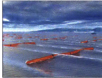
(b) Artist view of a Pelamis farm (attenuator devices) (Drew, Plummer, and Sahinkaya, 2009)
