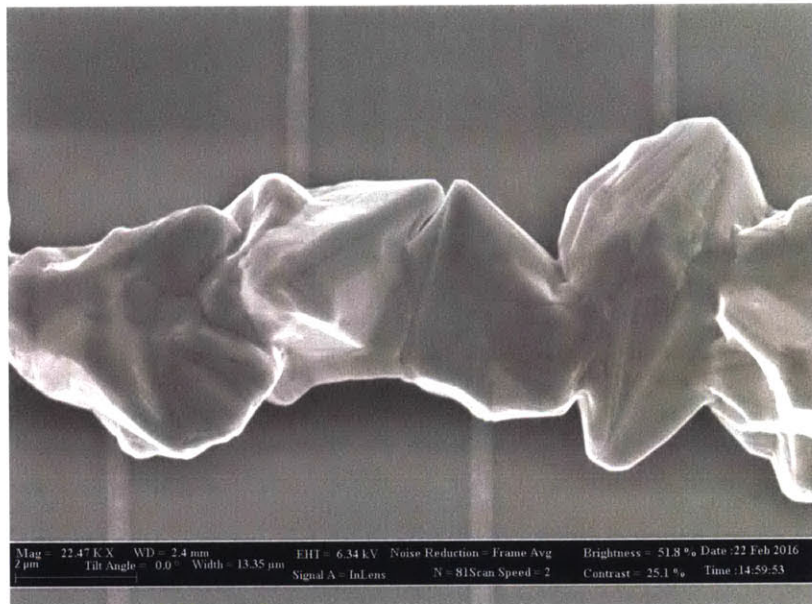
(b) Additional SEM image of a trench filled with coalesced Ge grains on SiO 2 utilizing the 2D GCLG technique.
