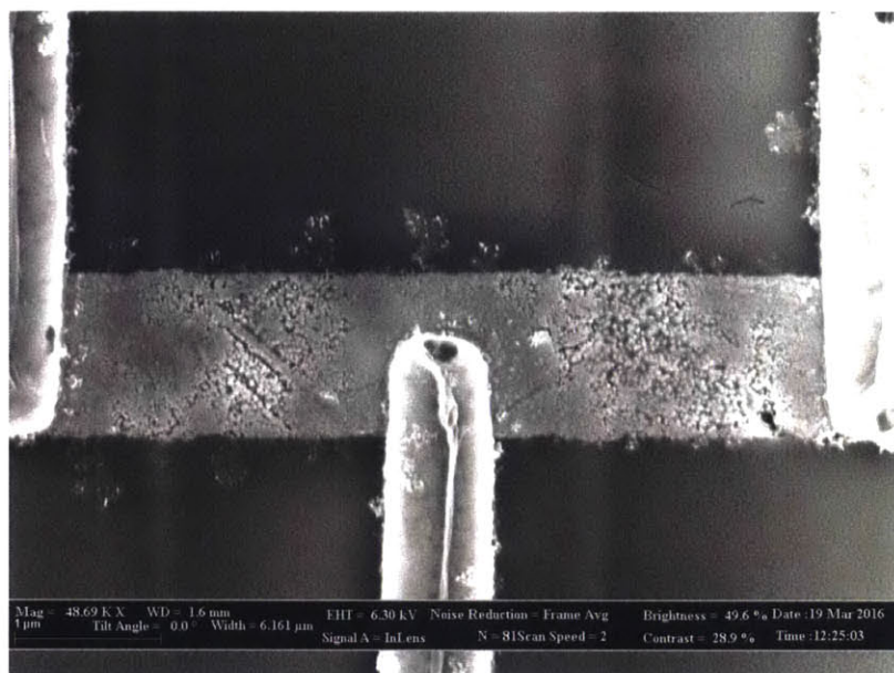
Figure 5-15: Plan-view SEM of final detector. Moderate surface damage is seen on the Ge surface due to overly aggressive chemical cleaning.
