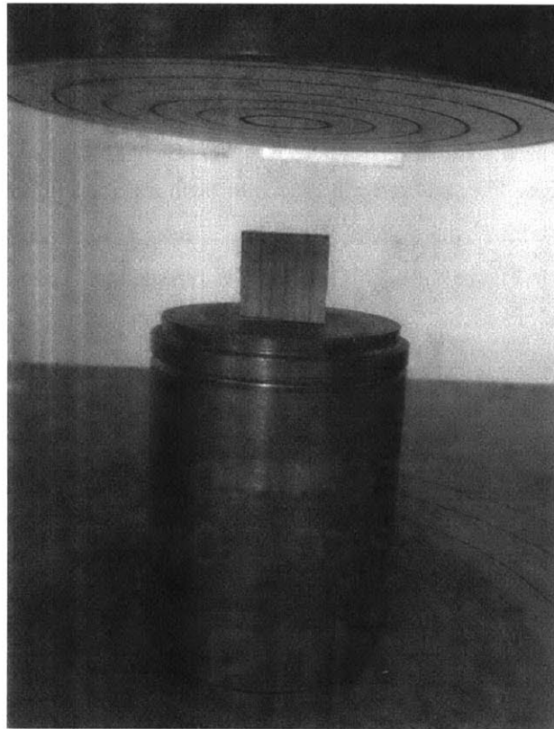
Figure 3-15. Clear wood test for compressive strength parallel to the grain of the wood
