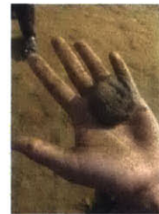
THE SOIL, CALLED "ROSHANI MITTI" IS USED TO MAKE THE FORMWORK. IT CONTAINS GOOD AMOUNT OF SAND AND SILT AND LESS AMOUNT OF CLAY.
