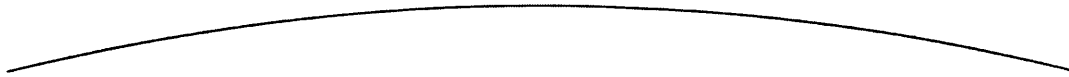
Figure 2.9: Parabola overlaid on catenary overlaid on circular arc for X = 12' , z = 9'' . The three curves are indistinguishable at this scale. After Allen and Zalewski (2010).
