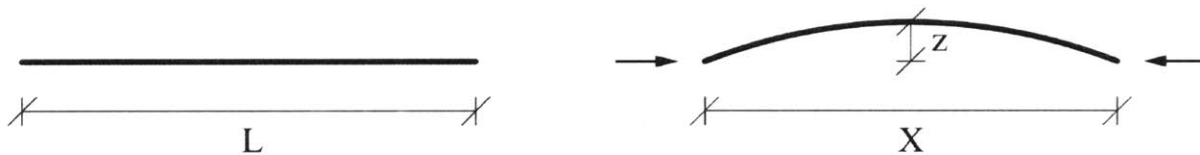
Figure 3.1: Elastica method for generating dome guidework
