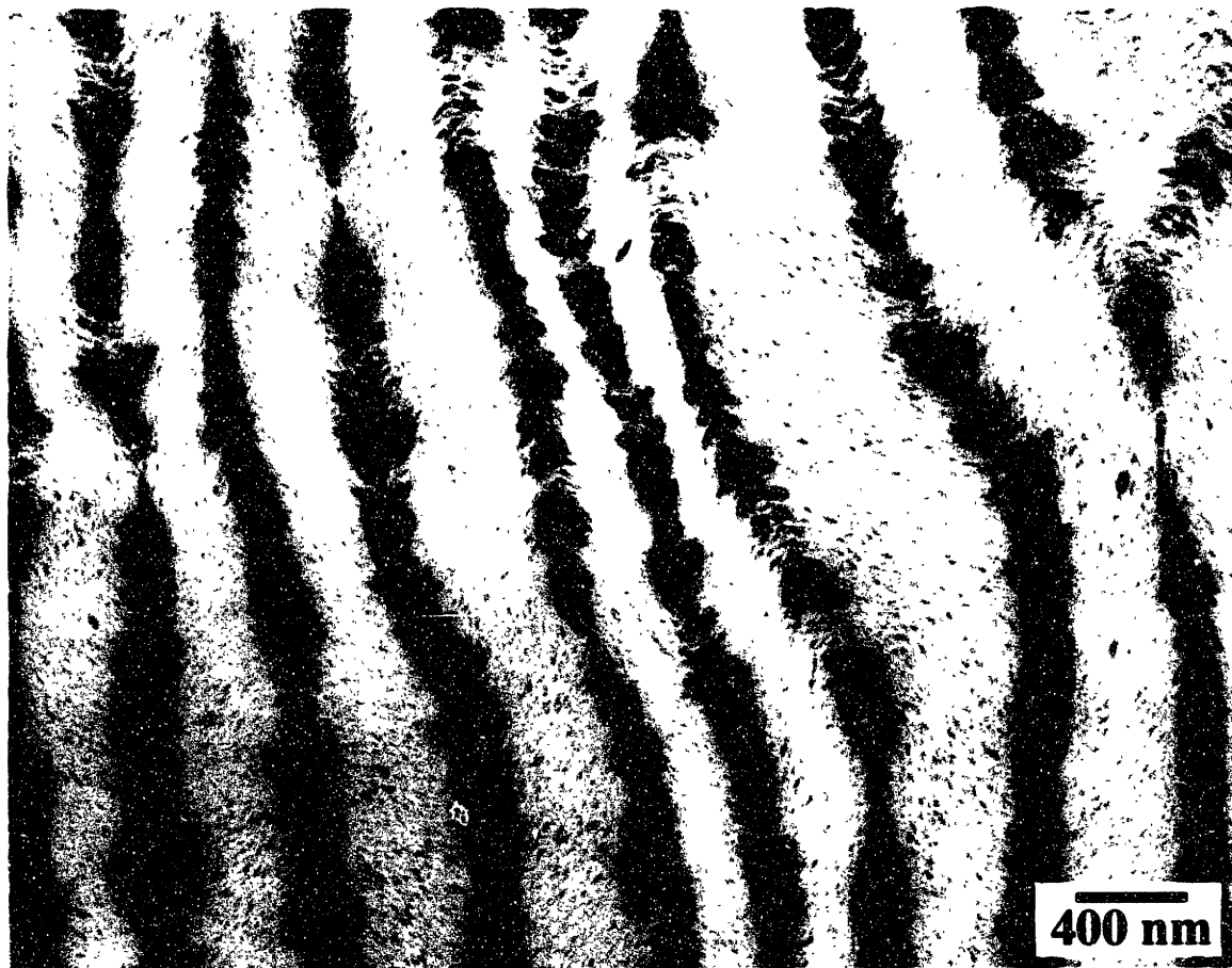
Figure 3.13 Bright-field TEM micrograph of HS245/9 which shows the variation in domain size observed in some areas of the sample caused by polydispersity. The light and dark regions are the PHIC and RuO 4 stained PS domains, respectively.
