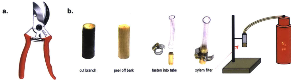
Figure 3-1: a) Corona pruner used for harvesting branches b) Steps involved in constructing a xylem filter [3]
