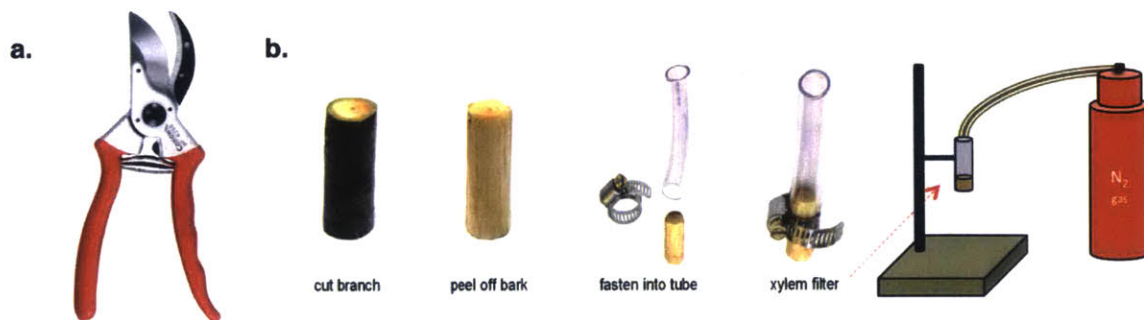
Figure 2-4: a) Corona pruner used for harvesting branches b) Steps involved in constructing a xylem filter [1]
