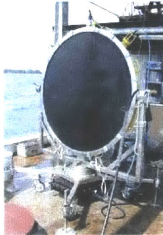
Figure 2-4: Remotely Operated Mobile Ambient Noise Imaging System, developed by Acoustic Research Laboratory (ARL) at the Tropical Marine Science Institute under the National University of Singapore [19].
