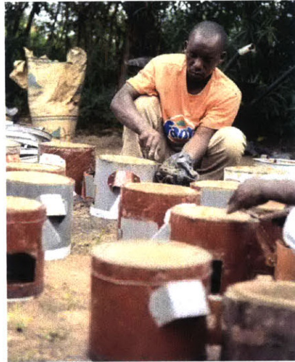
Figure 8: Artisan constructing a Makaa Stove
