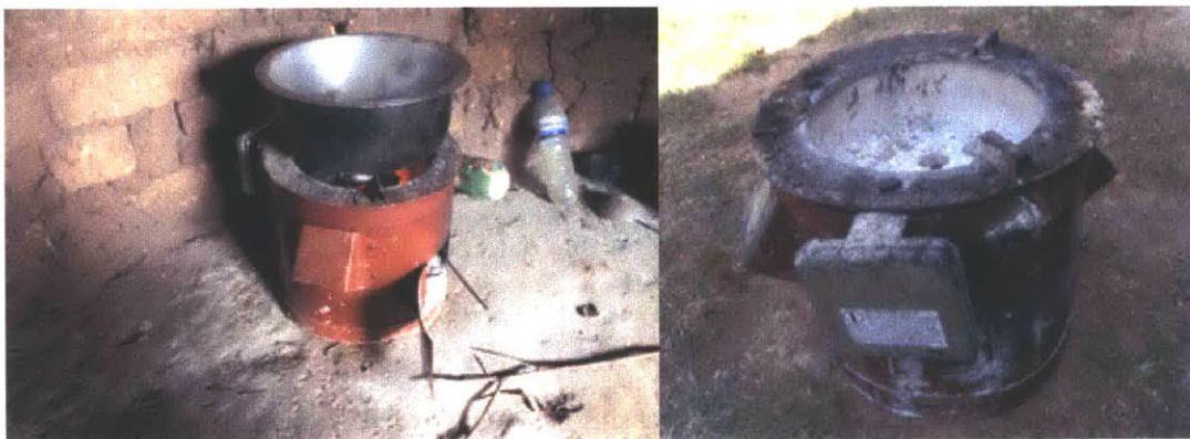
Figure 10: Examples of Sensen SUMs attached to AEST Makaa stoves
