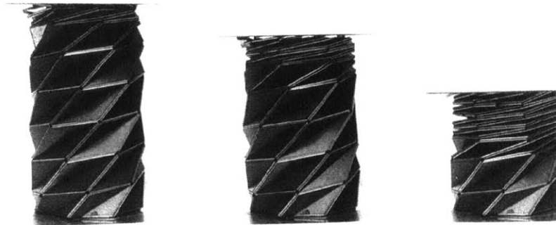
Figure 1-3: Folding sequence of triangulated cylinders from the work of S.D. Guest and S. Pellegrino [9]
