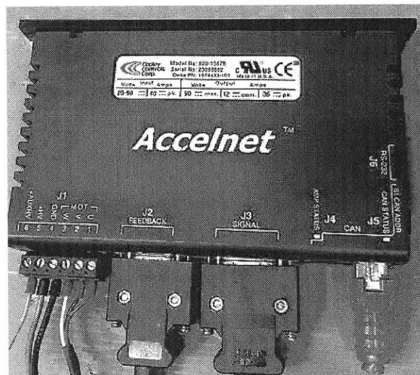
Figure 5-13: Copley Controls Accelnet panel chosen to control and drive the Parker actuators.
