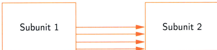
Figure 1-26: Two blocks with four connections between them. To save space and time the connectors could be drawn in a group, as in Figure 1-27
