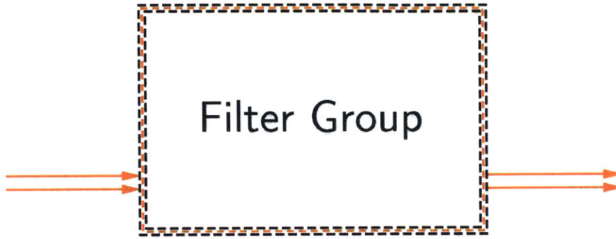
Figure 1-21: A collapsed version of a group with two inputs and two outputs.
