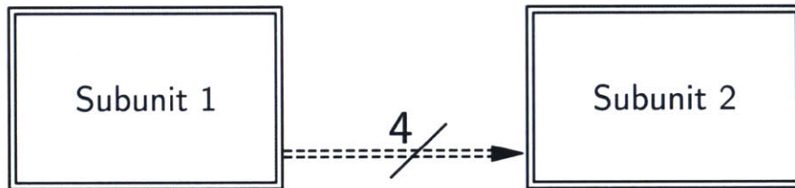
Figure 1-28: Two block prototypes connected by a group of 4 prototype connectors.
