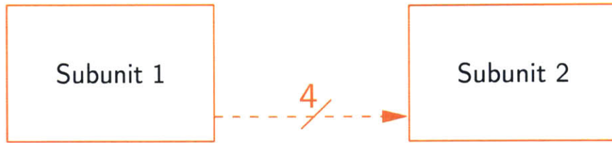
Figure 1-27: Two blocks with a group of connectors between them. Equivalent to Figure 1-26
