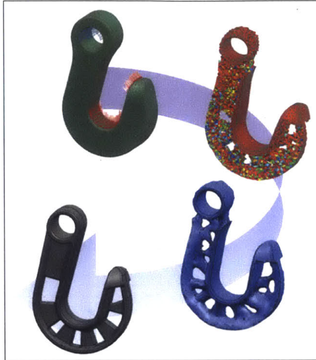
Figure 3-1: Design Steps in Topology Optimization (Siemens PLM Software, 2011). From upper left, clockwise: (1) functional structure definition (2) finite-element analysis of loads (3) component redesign to minimize volume (4) normalization of design for manufacturability.
