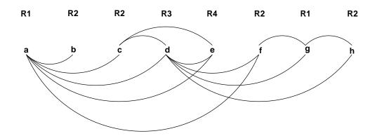
(b) Color your graph using as few colors as you can. Call the computer's registers *R*1, *R*2, etc. Describe the assignment of variables to registers implied by your coloring. How many registers do you need?
