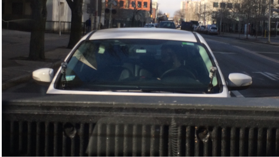
Figure 5-17: Chase Car with LIDAR and Sonar Mounted on Windshield Near Side Mirrors
