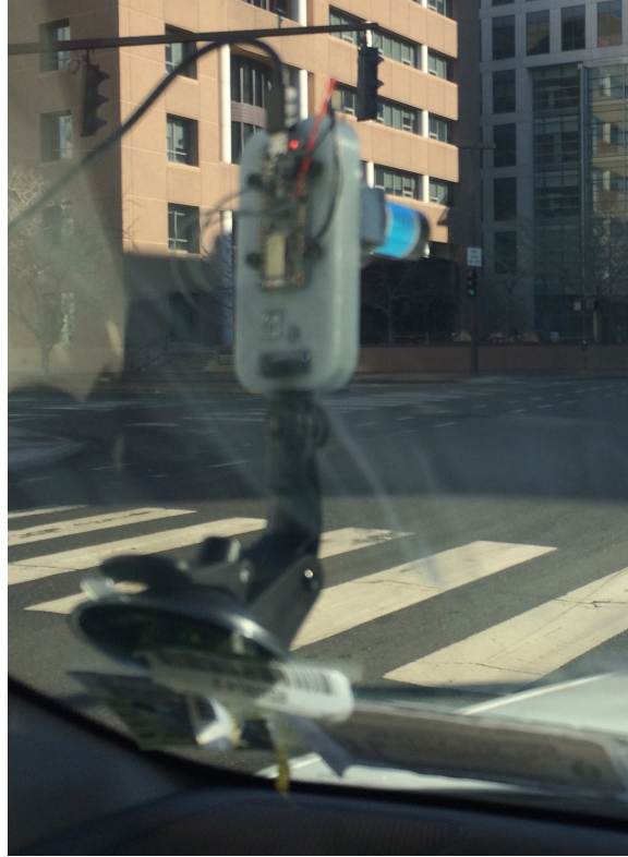
Figure 5-16: Windshield Mounted LIDAR and Sonar Rig (1 of 2)
