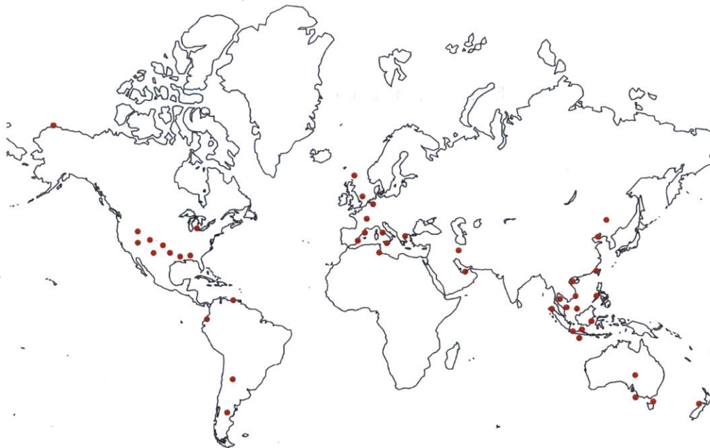
Figure 2. Global distribution of high (>20%) CO 2 -content basins and major developed natural CO 2 production fields (Adapted from: Baines and Worden, 2004; Stevens et al. , 2001; NETL, 2010). No data available for Canada and Russia.
