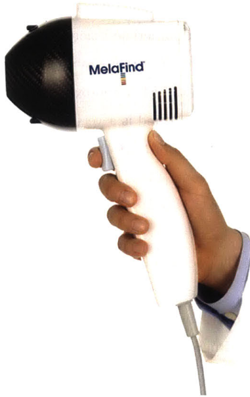
Figure 3-4: MelaFind – a multi-spectral imaging system for melanoma diagnosis [131]
