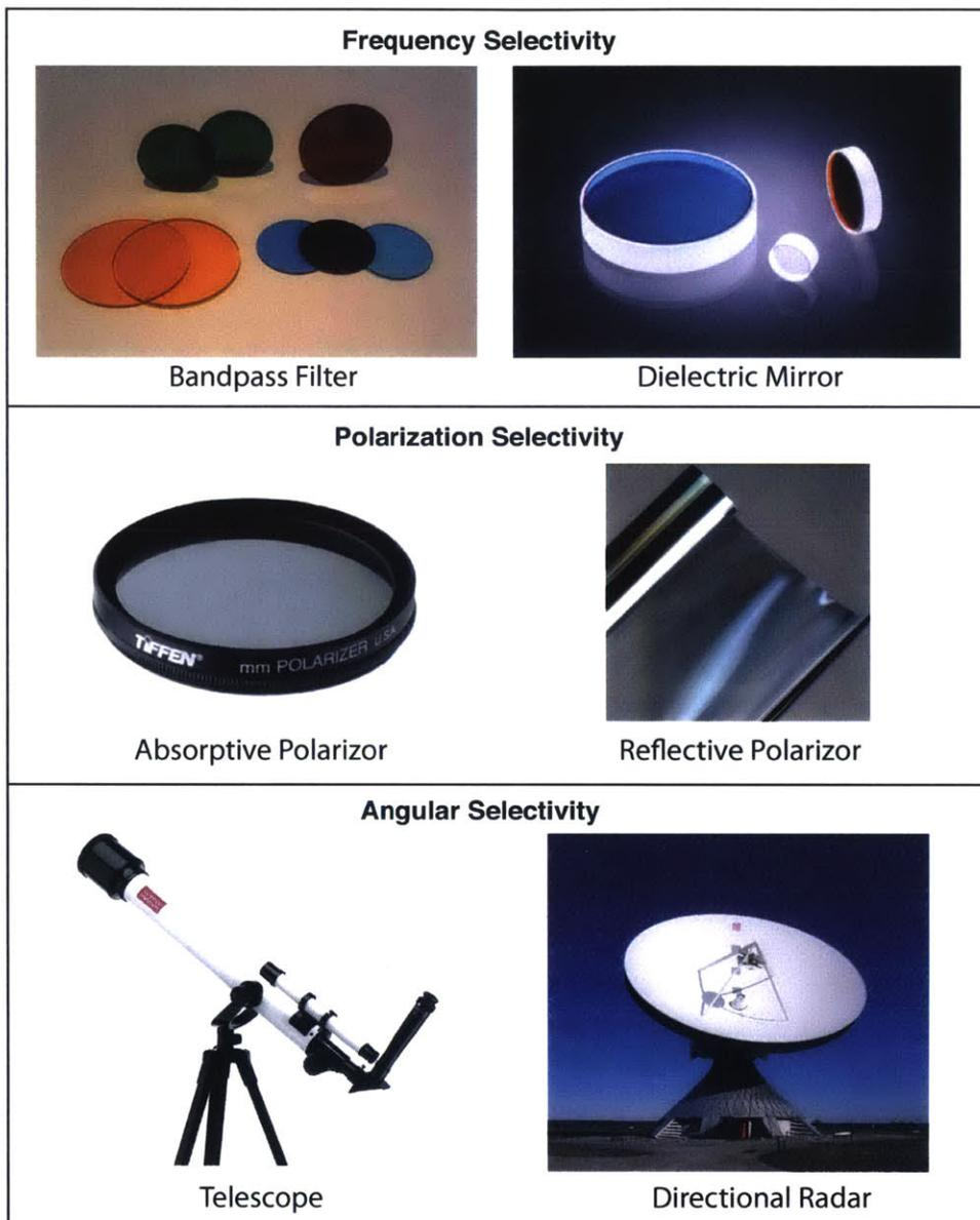
Figure 2-1: **Conventional light selective devices.** Frequency selectivity can be achieved by bandpass filters [15] or dielectric mirrors [16] (top panel); Polarization Selectivity can be achieved by wire grid polarizer, polaroid (polyvinyl alcohol polymer impregnated with iodine), or multilayer materials (3M Inc.) [17]; Traditional angularly selective devices are mainly based on geometric optics, such as telescopes [18] and radars [19].
