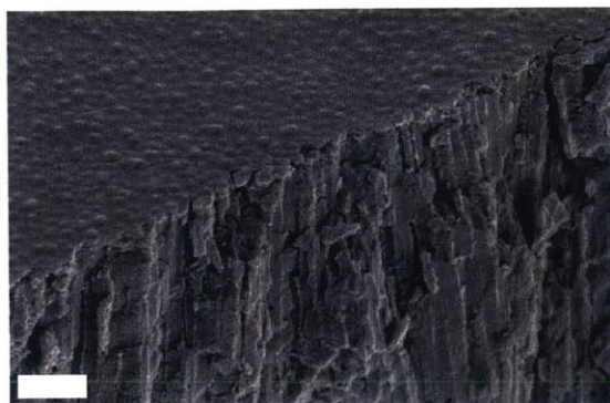
Figure 13: Cross section SEM image of a membrane filled with photoresist, showing pores completely filled up to the membrane surface. (scale bar: 1 \mu\text{m} )
