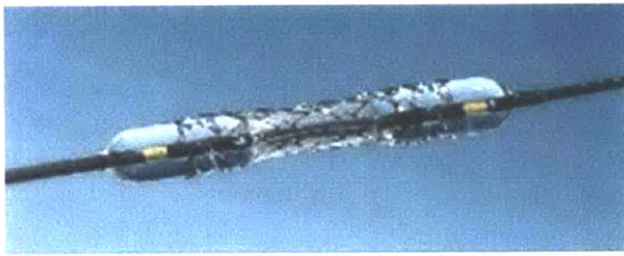
Figure 3-1 Specially-modified balloon catheter To create underexpansion of the stent, the balloon catheter is restricted from its full expansion by placing a PET tube, whose diameter is smaller than that of the balloon catheter, over the balloon catheter in the middle region.
