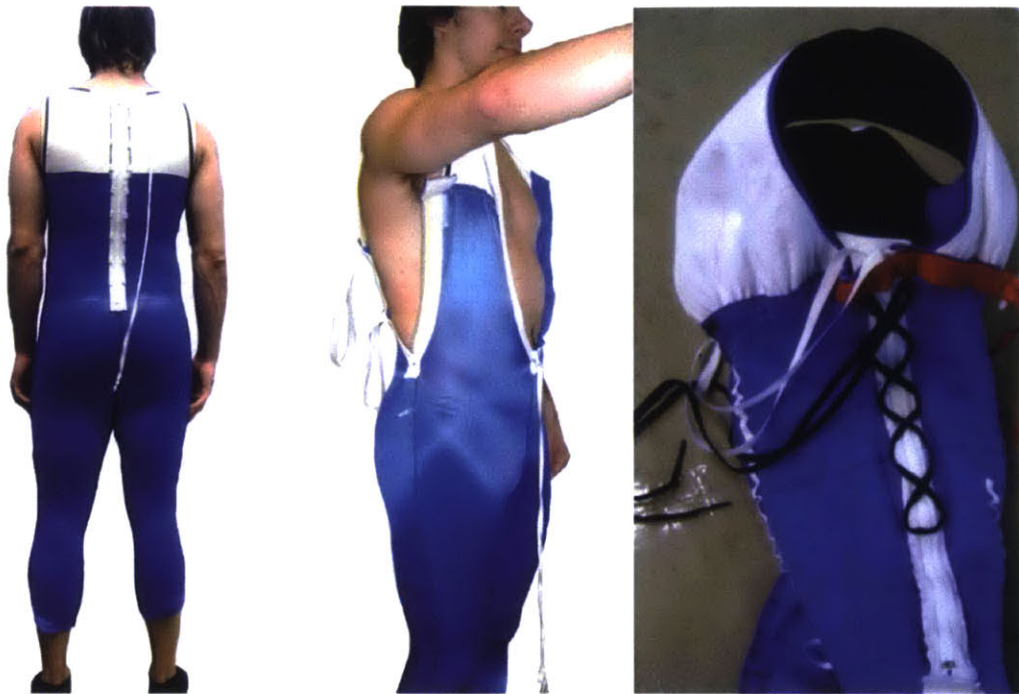
Figure 1-5: GLCS Mark IV suit: (L-R) Back Zip, Side Zip, and Side Zip Lacing
