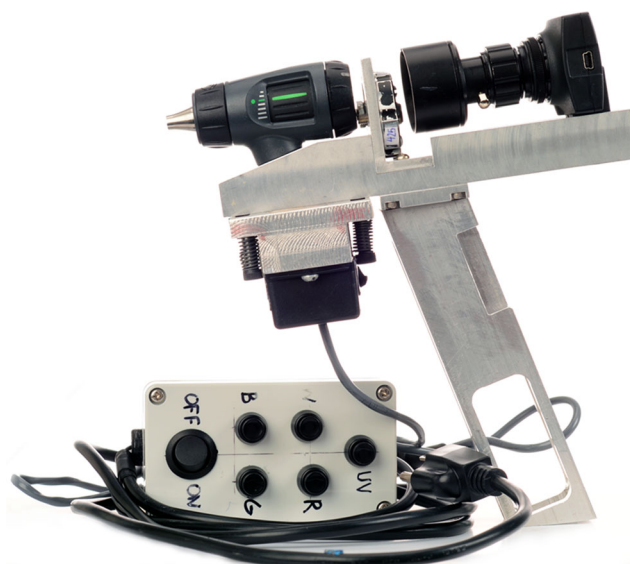
Fig. 1 Photograph of the modified otoscope prototype with sequential white-light examination and narrow-band reflectance imaging capabilities. This prototype system was used in the human subject pilot study to evaluate the potential of the multi-wavelength reflectance imaging approach in evaluating middle ear pathological conditions
